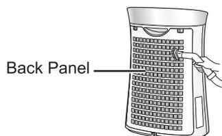
Gently remove dust from the back panel by using a vacuum cleaner attachment or similar tool.
