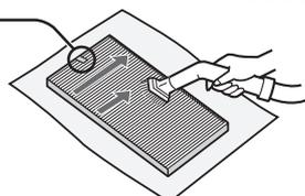
Gently remove dust from HEPA Filter and Deodorizing Filter with a vacuum cleaner attachment or similar tool.
