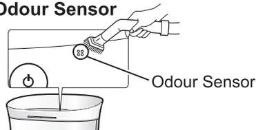
Gently remove dust from the Odour Sensor by using a vacuum cleaner attachment or similar tool.
